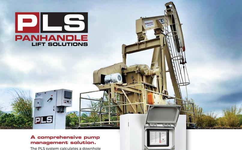
The PLS system calculates a downhole card by solving the 1D wave equation using the directly measured surface load and position as the initial boundary conditions.
